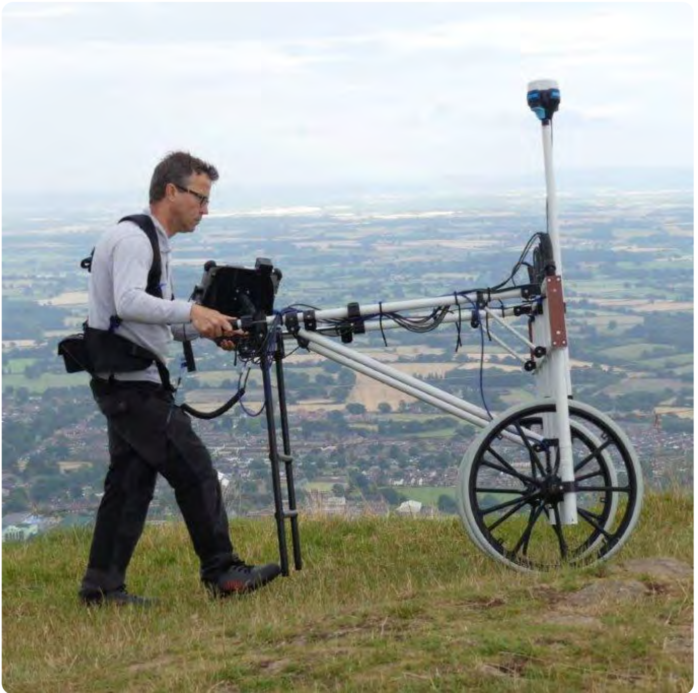
Data Collection with a magnetometer, Malvern Hills.
