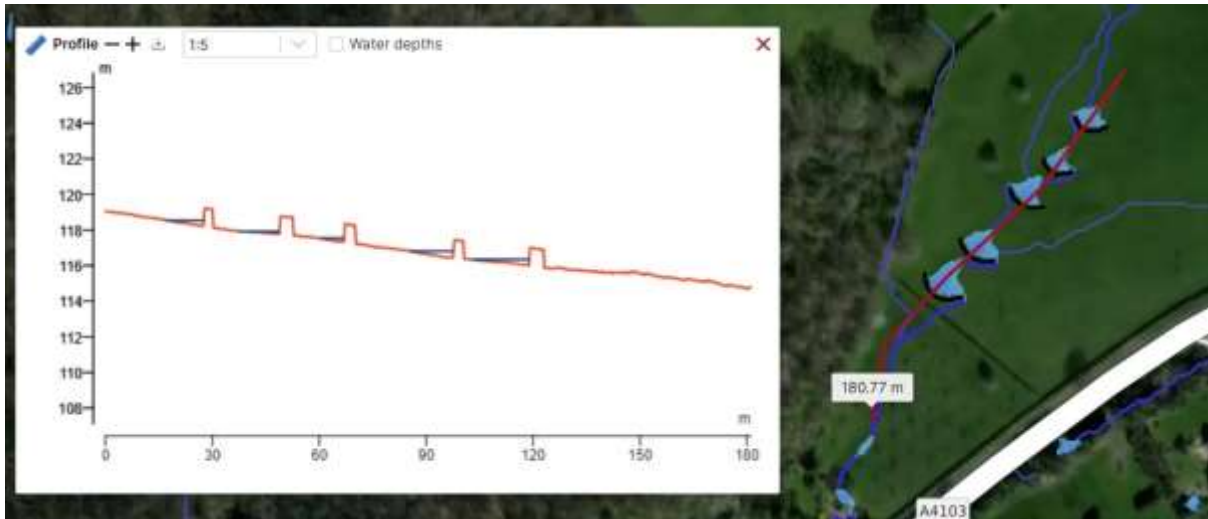
Figure 42 Cross section of grass bunds on aerial photography at Case Study 1 (SCALGO 2025)
