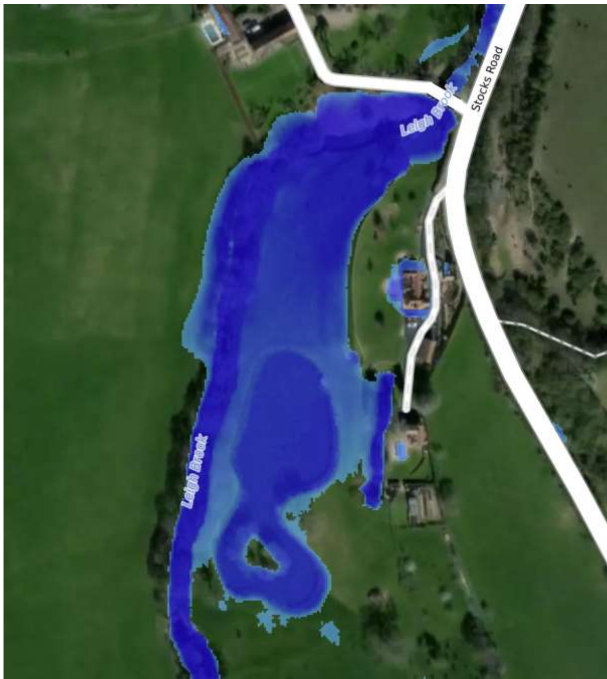
Figure 80 Modelled standing water at land near Stocks Road (SCALGO 2025)
