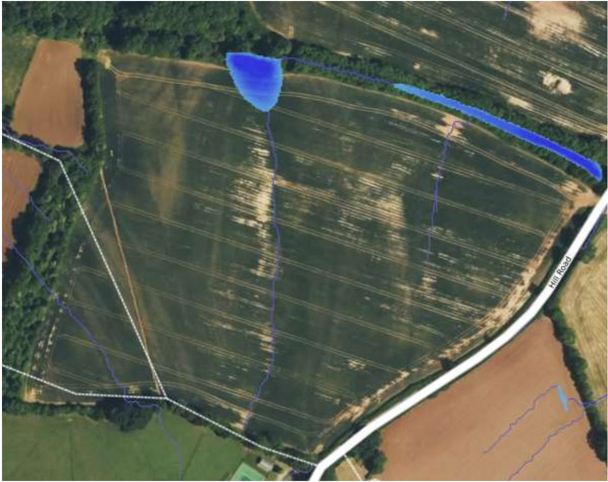
Figure 69 Significant overland flow pathways modelled using SCALGO are in the same location as the rills/gullies seen in 2013 and 2017 (SCALGO 2025)
