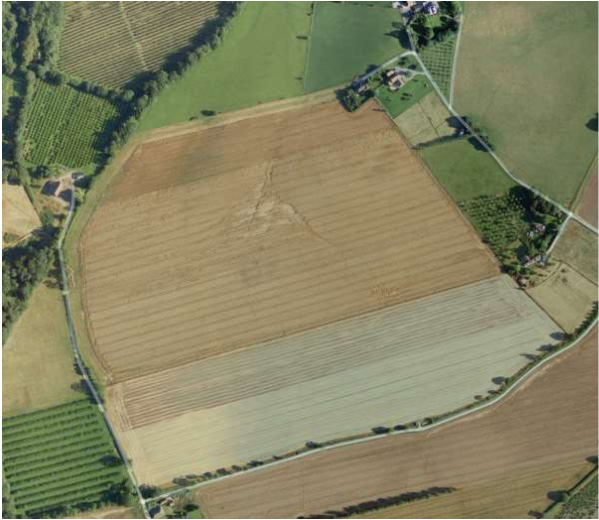
Figure 71 Evidence of soil erosion (rills/gullies present) in aerial photography (Google Earth 2025)
