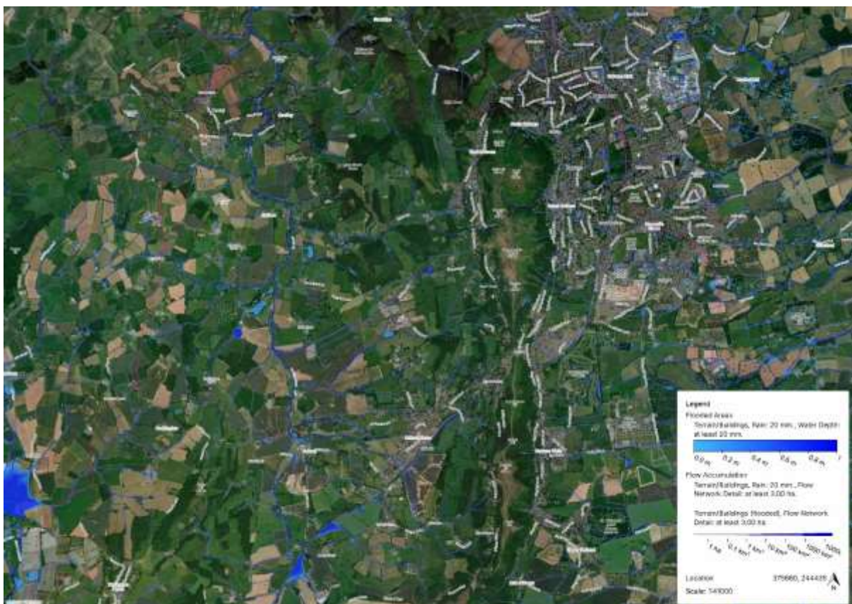
Figure 23 MHNH overland flow pathways and water ponding (central) (SCALGO)
