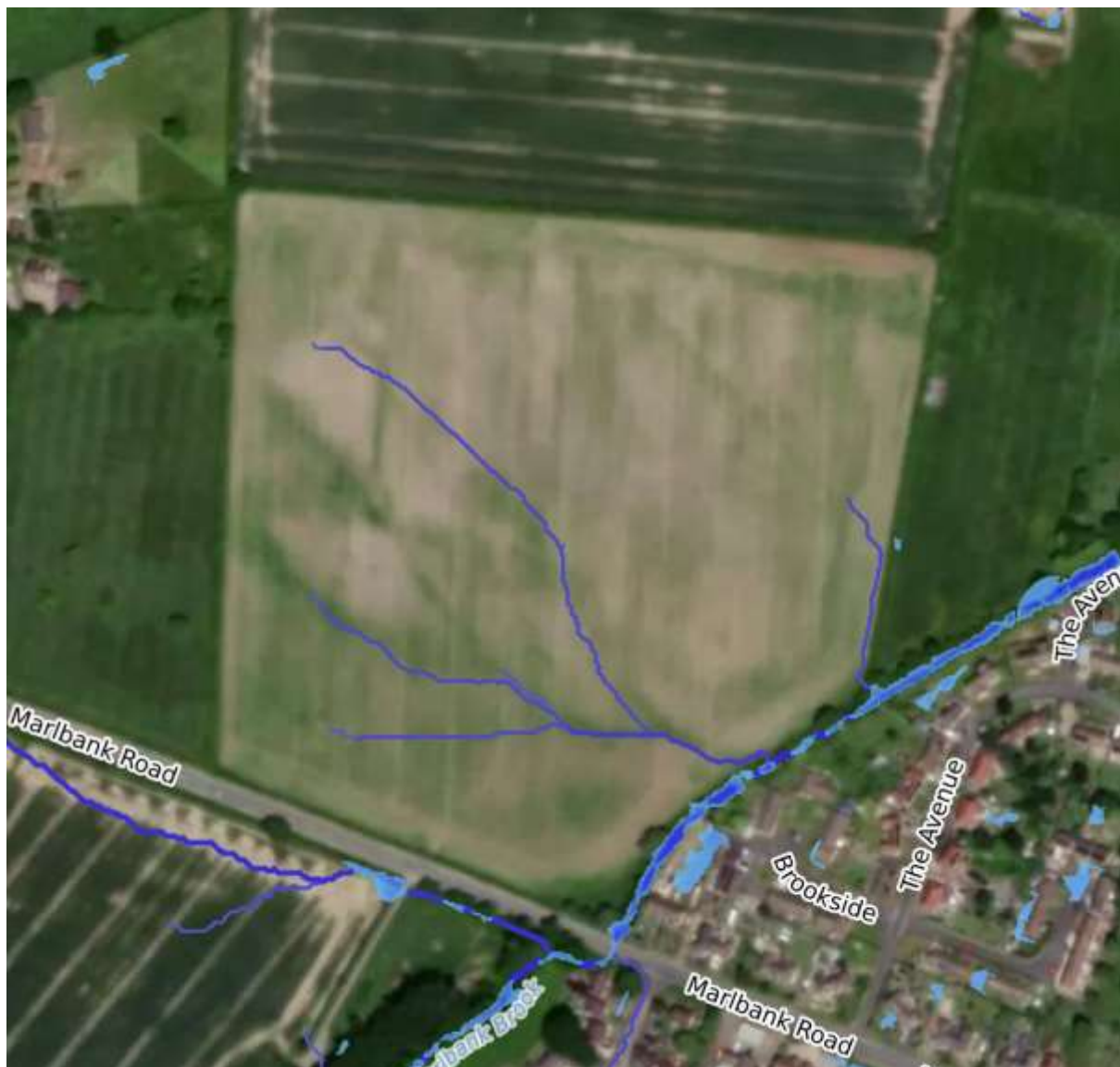
Figure 95 Modelled overland flow and flooded areas over areal photography at site 16 (SCALGO 2025)
