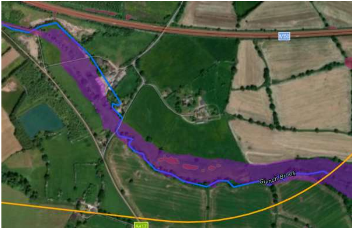
Figure 111 WWNP Runoff attenuation features 3.3% AEP for potential pond at site 22 and Flood Zone 2 (WWNP 2017)
