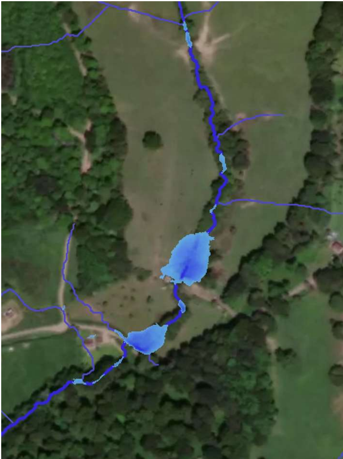
Figure 104 Modelled overland flow and flooded areas at site 20 (SCALGO 2025)
